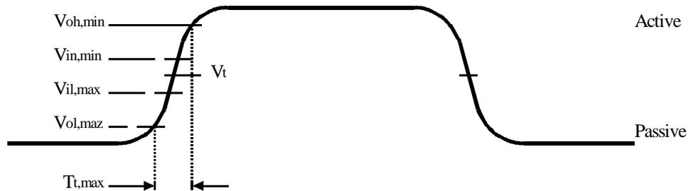
Figure 9. SAE J1850 VPW Waveform
